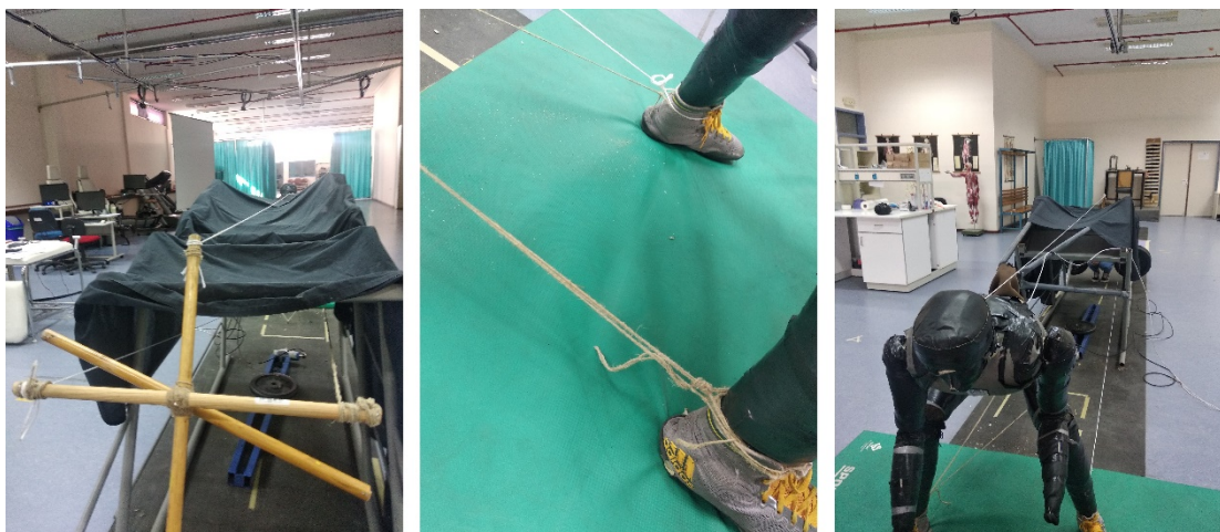
Figure 2. Wooden construction and connection with the dummy's legs
